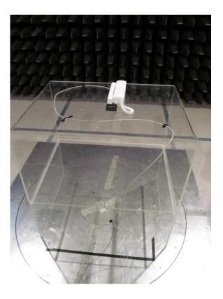
Test location: EUT to antenna distance: Operation mode: Limits: semi anechoic chamber 3 m active
